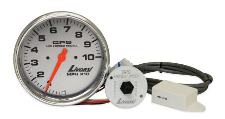
Livorsi GPS Speedometers are more accurate than ever with the optional GPS antenna with a 10X update. What does this mean? It means your GPS Speedometer will show your true speed faster because the antenna updates 10 times per second eliminating pointer lag.
